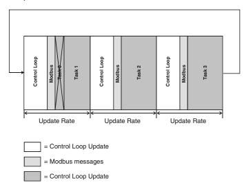
Figure 108: Time Slicing Diagram (Task 0 blocked)
